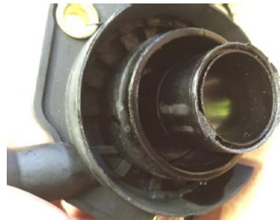
Off Axis Wear On Guide Tube
