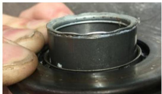
Damaged Piston Stop
